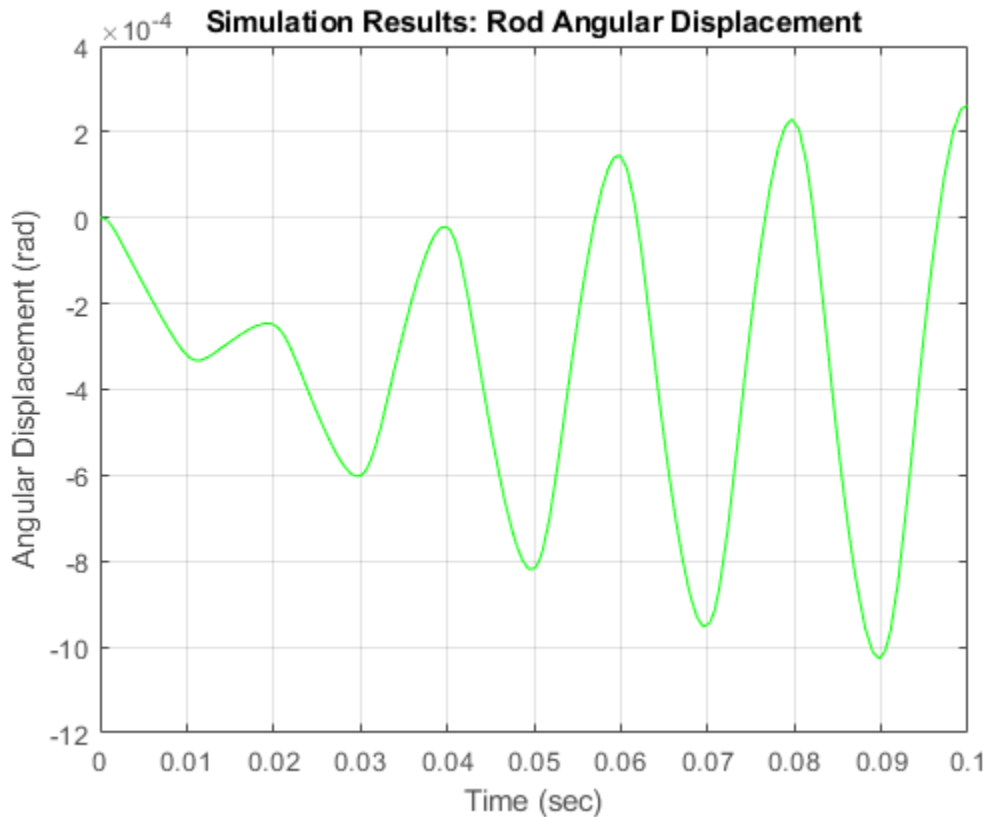
Figure 4: Angular displacement of the rod
